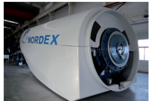
Assembly of wind turbine generator
