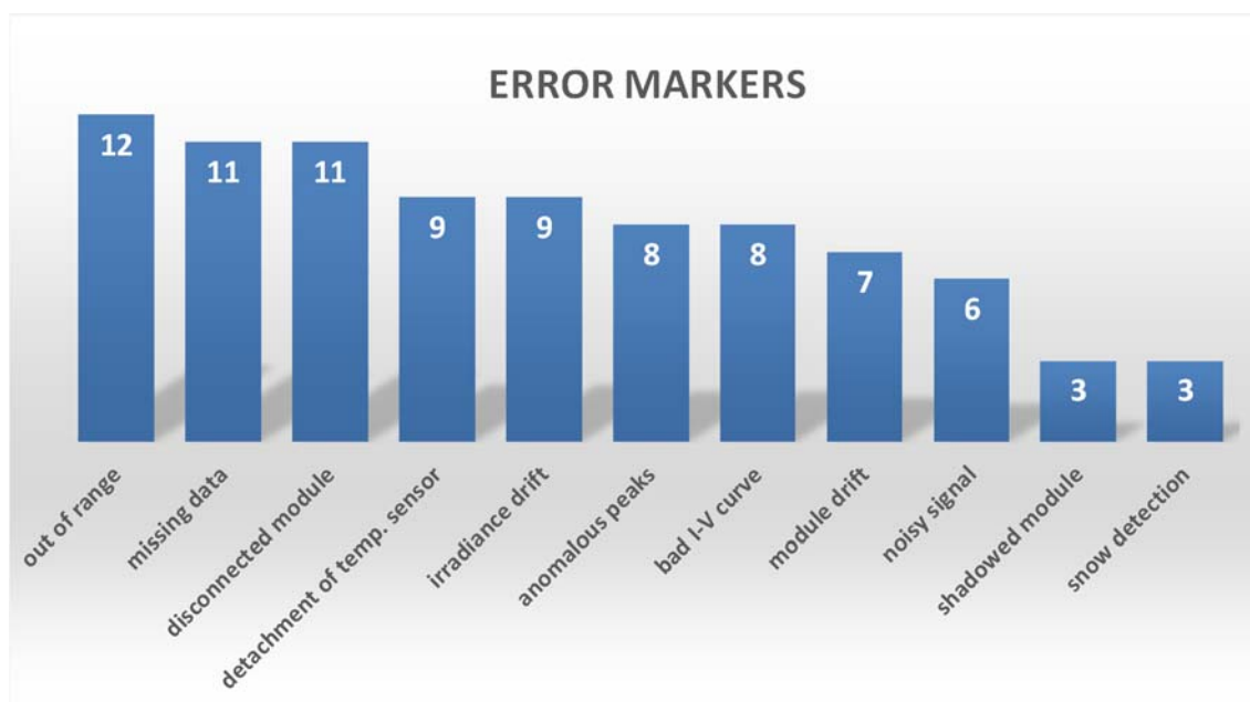
Figure 22: Type of data quality controls (error markers) and the number of laboratories implementing them.
