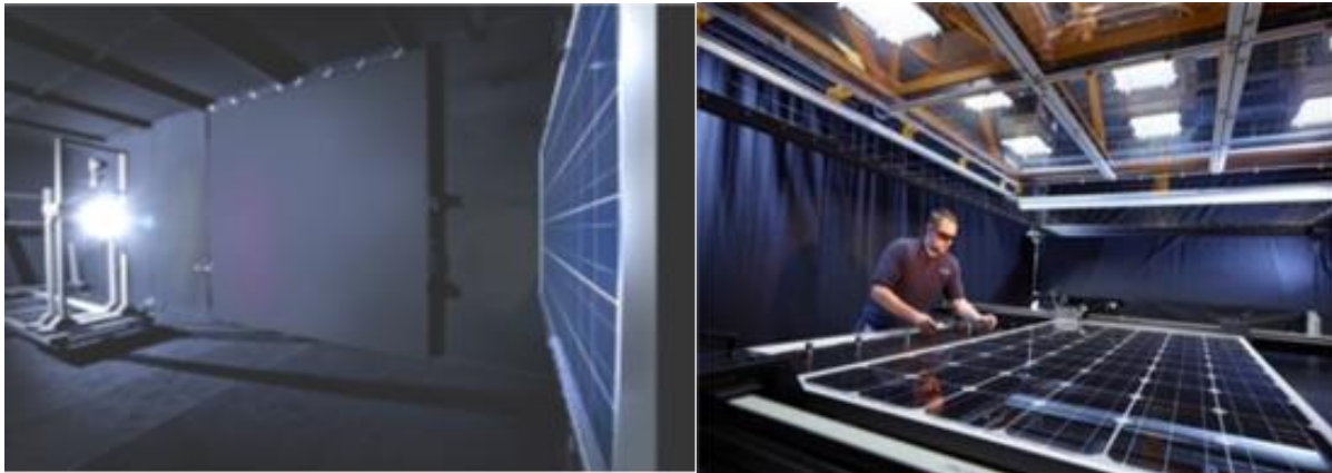
Figure 5: Solar simulators for PV modules, left: pulsed, right: steady state (Source: TÜV Rheinland Group).
