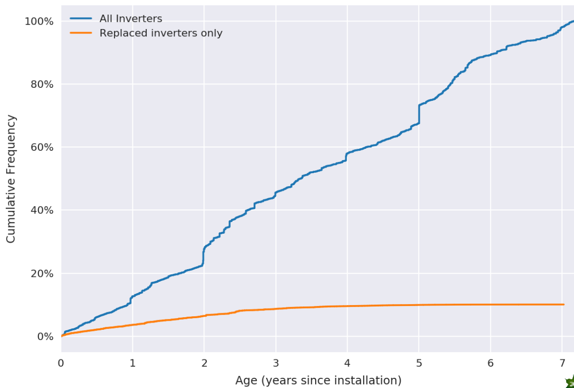
Figure 24: Cumulative distribution function of inverter operational lifetime (total population: 40955 inverters; source: 3E SynaptiQ monitoring system)
