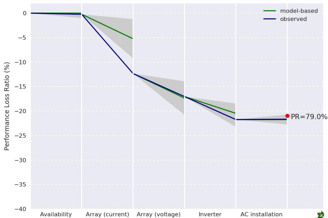
Figure 27: Waterfall diagram of Performance Loss split over the energy conversion chain (example)
