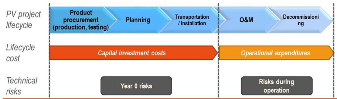
Figure 1: Lifecycle costs of PV projects and the link to different project phases
