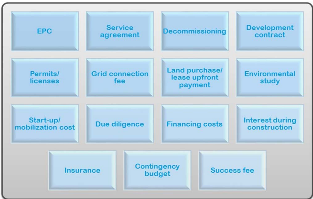
Figure 6: List of CAPEX items found in surveyed financial models of ground mounted PV projects in FR and UK
